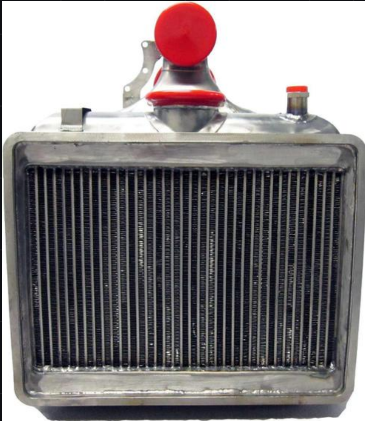
F-15 PRIMARY HEAT EXCHANGER · FIN &amp; PLATE
